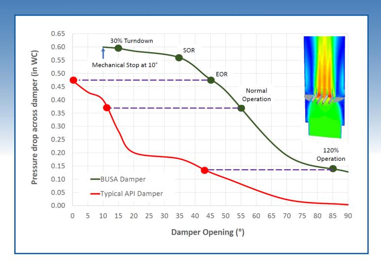
Linear controllability through an expanded range is of critical importance when automation of the heater combustion is the goal, especially when the targeted excess O2 is at levels of 3% or less.
